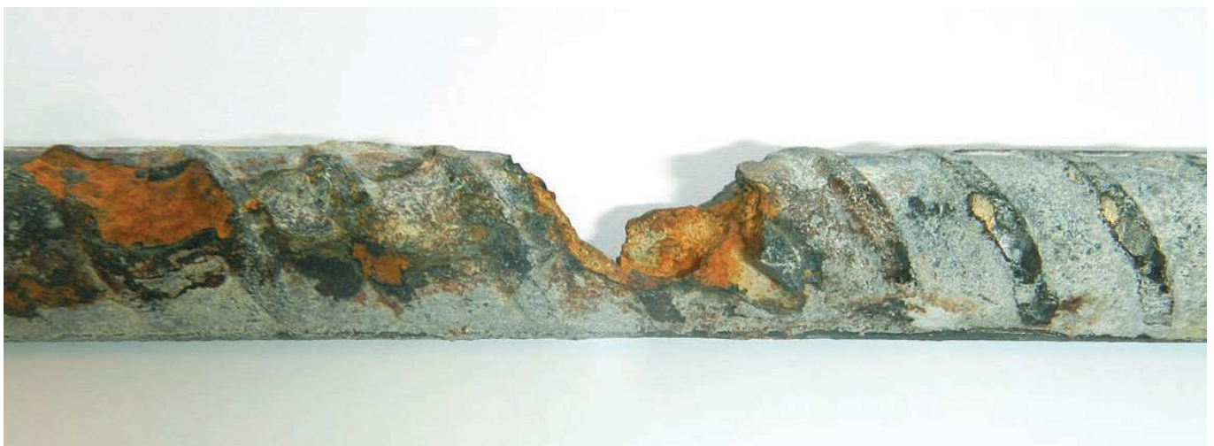
Fig. 2: Typical pitting corrosion
