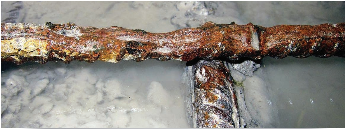
Fig. 1: Cross section reduced by corrosion
